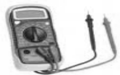
Meter to test heater & sensor after 3 fitting
