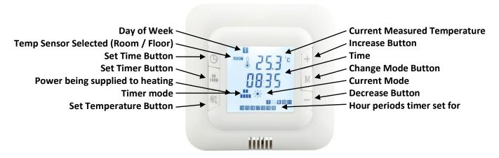
Please note: Whilst programming, if nothing is pressed for 5 seconds, the thermostat will return to main screen.
