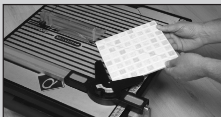
Re-tighten the knob and position the tile within the jaws of the Mitre Guide.
