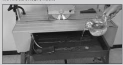
Ensure that the drain plug is in position, then fill the water tray until the pump is almost submerged (approx. 10 litres). Check water level regularly and top up as necessary. Do not allow pump to run dry.
