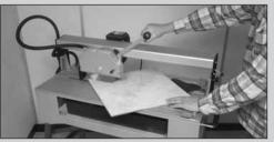
Pull the blade carriage steadily towards you, cutting through the tile. When the cut is complete, switch off the machine, removing the cut tile pieces and any debris.
