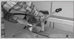
Whilst holding the shaft with the spanner wrench, turn the blade retaining nut clockwise to release using the hex wrench.
