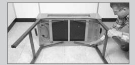
Remove the saw from its carton, lay carefully on its side. Pull down the legs and fasten the four support brackets to them using the nuts provided.
