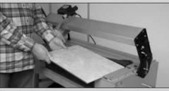
Place the tile in position on the cutting table so that it rests against the measuring scale and the mitre guide. Switch on the machine.
